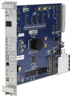
• The GTWIF provides the communication interface between the Local Area Network (LAN) and the RTDS Simulator. Each GTWIF is assigned a unique IP address so that it may communicate with any computer or device accessible on the LAN.
